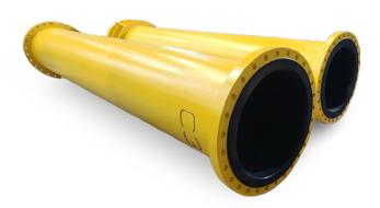
RMB provided a 100% corrosion protection system, including an HDPE liner, exterior topcoat, and polysulfide sealant to address vulnerabilities at material interfaces. The polysulfide sealant, a technology transfer from RMB's aerospace division, was particularly crucial in sealing the small gap between the liner and the exterior coating, preventing corrosion in this vulnerable area that will be exposed to the corrosive seawater.
