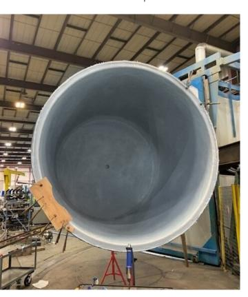
ETFE's excellent chemical resistance properties supply longterm protection against the harsh processing environments the tank encounters. The mechanical bond between the lining and substrate enables better management of thermal expansion, reducing stress on the lining during temperature fluctuations.
