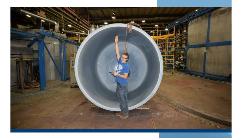
Large-Scale Rotational Lining for Chemical Processing Equipment
