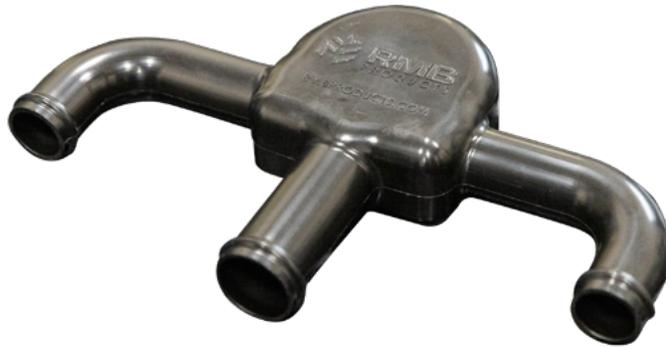
Next, during the cooling phase, the melted polymer solidifies, maintaining the shape of the mold. The resulting piece is seamless, devoid of any weld lines or joints. This method offers several advantages, including part flexibility, to deliver a durable, lighter-weight solution compared to a similar metal part. In addition, this process minimizes waste to help companies meet sustainability goals.
